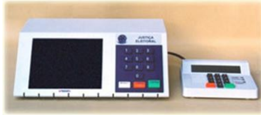
Fig. 1. The BEVM and the micro terminal used by poll clerk to control voting sessions.
